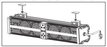
4. Dermine the size of the bar and then select the appropriate size clamp ring. The XBAR offers a 1.75" and a 2" clamp ring (parts list nos. 7 and 8) to fit bars from 1.5" to 2". Refer to the chart below to select the appropriate size clamp ring.
