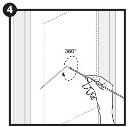
Fold a coat hanger or other sturdy metal piece of wire, bend it 90°, and insert it into the pilot hole as shown above. Rotate the wire 360° to ensure here are no obstructions.
