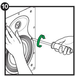
a drill or phillips head screwdriver, turn each one of the mounting screws clockwise until the clamps firmly grip the wall. Now tighten each screw one additional turn to ensure that the clamps are locked in. Do not overtighten.
