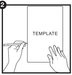
Position the cutout template and use a level to ensure that it is properly aligned. Use a pencil to trace around the template and recheck the tracing to make sure it's level.
