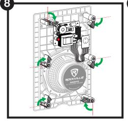
Make sure the mounting screws are in the locked position. If they are not, turn them a quarter turn counterclockwise until they stop.
