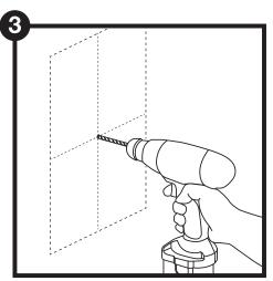
Use a ruler to locate the center of the outline you traced and drill a pilot hole there.
