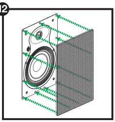
The grill is secured to the speaker with magnets. Simply place the grill on top of the speaker until you feel it catch. As these grills are painteable, be sure to paint them prior to installation.
