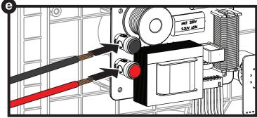
Warning: Make sure that the positive (+) and negative (-) speaker wires are connected to the corresponding terminals on the speaker and the amplifier.
