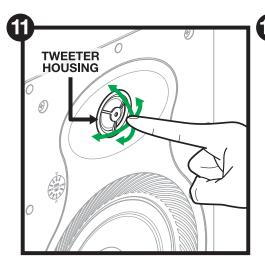
Once the speaker is mounted, you can adjust the angle of the tweeter to ensure it's pointing towards the listening position. Do this by gently pressing the outer edges of the tweeter housing as shown above. DO NOT PUSH ON THE ACTUAL TWEETER. Doing so will cause permanent damage.
