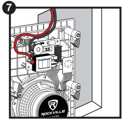
Connect the speaker cables to your speaker. Refer to the Setup section on the next page for detailed instructions.
