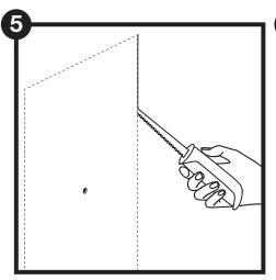
Use the drywall saw to cut out the outline you traced on the wall. Before cutting, check the outline to ensure that it is straight and level.
