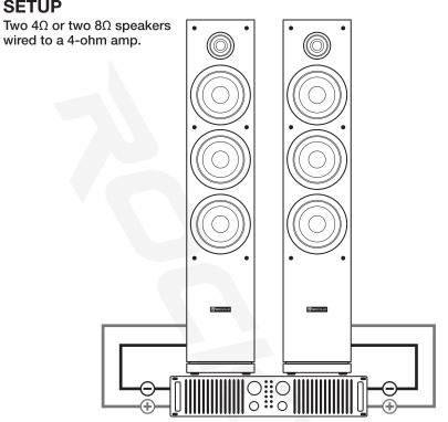
Two  $8\Omega$  speakers wired in parallel to each channel of a 4-ohm amp.
