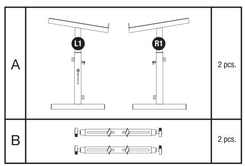
Begin by taking part B and loosening both extension lock knobs (fig. A). Extend both arms approximately 1 inch (the arms can be extended up to 23.6 inches). Tighten the lock knobs to hold the extension arms in place (fig. B). Do this for both nieces.
