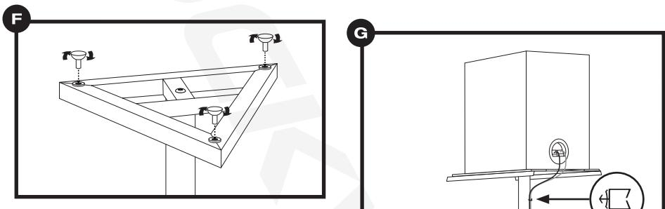
If you are placing the stand on a wood, laminate, tile, or bare floor you should use the included rubber feet. To install, simply screw them into the holes at the bottom of the base plate.
