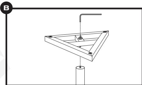
Turn the triangular base so that the insertion points for the rubber feet/steel spikes are facing up. Insert a long screw (removed from the telescoping shaft) and washer through the opening on the base and the opening in the shaft mounting plate. Push the plate against the base so that it fits snugly.
