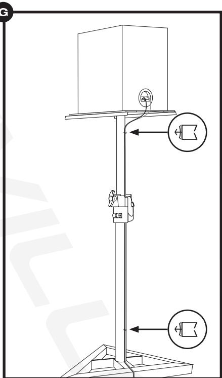
Finally, connect the cable clips to the small holes found on the rear of the stand. There is one just underneath the speaker platform and one near the base. Once they are in place, guide the speaker wires through the top clip, then along the telescoping shaft to the bottom clip. This will help keep the speaker cables tidy and out of the way.
