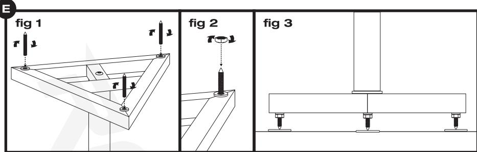
To place the stand on a carpeted floor, use the metal isolation spikes. Attach the spikes to the bottom of the base plate (fig 1). If needed, adjust the spike height to keep the stand level. Use the nut to secure the spike in the desired position (fig 2). Place a metal disk underneath each spike to protect the surface on which the stand is placed (fig 3).
