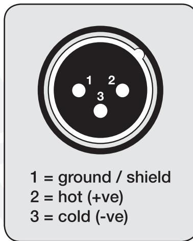
These microphones can be used for balanced and unbalanced applications. For balanced XLR connections use an XLR cable (not included). For unbalanced connections use a 1/4" TS jack plug to a female XLR cable (not included). Be aware that when using a run longer than 16ft you may encounter humming caused by stray magnetic fields from power cables, lighting cables, and other electric appliances.
