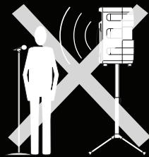
Feedback can also be caused by the acoustics of the venue. In these instances the proximity effect may cause feedback. In most cases, simply moving a little away from the microphone may resolve the issue.
