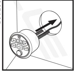
3. Slide the mounting bracket onto the unit as shown in the illustration. The bracket should sit firmly against the bolts and the arms should sit firmly against the mounting surface.
