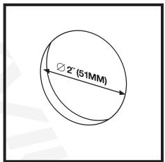
2. Feed the remote control cable into the hole and connect it to the included remote extension cable which should be connected to the remote control input on the RGHR45 receiver. Now slide the remote control unit into the hole until it sits firmly against the mounting surface.
