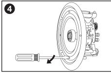
Screw down each of the four Phillips head screws. The locking tabs will swivel into place and secure the unit to the rear surface of the drywall. Put in the strips of adhesive to secure the grille.
