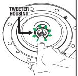
Use a Phillips head screwdriver to turn each screw clockwise. This will cause the locking tabs to swivel into position. Continue turning each screw clockwise until you feel resistance, securing the unit to the back surface. Adjust the angle of the tweeter to ensure it's pointing towards the listening position. Do this by gently pressing the outer edges of the tweeter housing as shown above. DO NOT PUSH ON THE ACTUAL TWEETER. Doing so will cause permanent damage.
