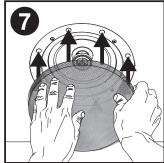
Place the grill over the speaker and listen for the sound of the magnets connecing to it indicating that it is securely attached. Once mounted, tweeter attennuation can be adjusted by taking the speaker out or physically adjusting the tweeter.
