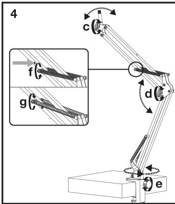
To adjust the position of the microphone (fig. c), adjust the angle of the boom arm (fig. d), or to rotate the boom arm (fig. e): loosen the corresponding knob, make your adjustments, then tighten the knob. Do not overtighten.
