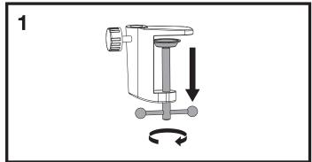
Turn the metal handle clockwise to open the clamp.
