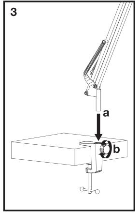
Insert the boom arm assembly into the corresponding opening on the clamp (fig. a). Turn the knob to secure the boom arm assembly (fig. b). Do not overtighten.
