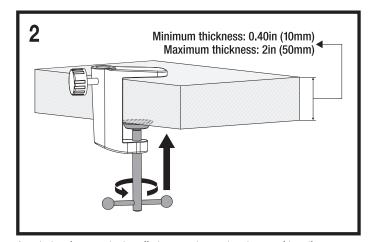
Attach the clamp to the installation area by turning the metal handle counter-clockwise until the bottom of the clamp is tightly secured.
