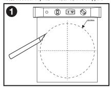
Using the included template, cut an opening in the ceiling.
