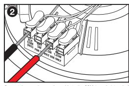
Connect the negative speaker cable to the COM (negative) terminal and the positive speaker cable to the appropriate 70 volt terminal.
