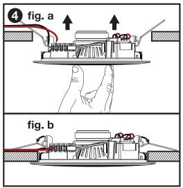
Once the retainers have cleared the opening, release them. Continue pushing the speaker until it is flush with the ceiling. The retainers will snap down to hold the speaker in place.
