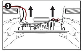
Push and hold the spring-loaded metal retainers on either side of the speaker and insert it into the opening.
